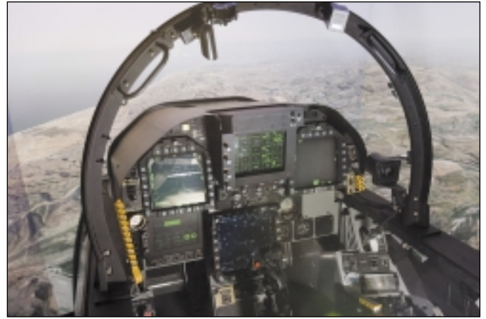
Boeing used the show to launch a new high-resolution faceted display system using curved facet screens and HD projectors.
