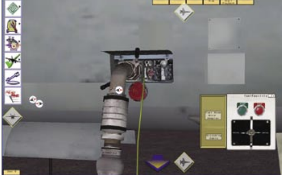
Virtual training and familiarization marries high-fidelity models with on-screen assistance as seen here with the refuel/defuel panel and the fuel facility displayed for easy user interface as well. [DiSTI image]
